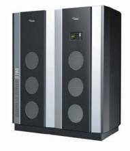
Two independently usable GS units, each with a capacity of max. 64 Gbytes as well as remote installation (max. 70 m), increase the fail-safe aracteristics of high-speed memory. The GS units are directly connected to the computer-internal memory control unit via fiber-optic cable.
